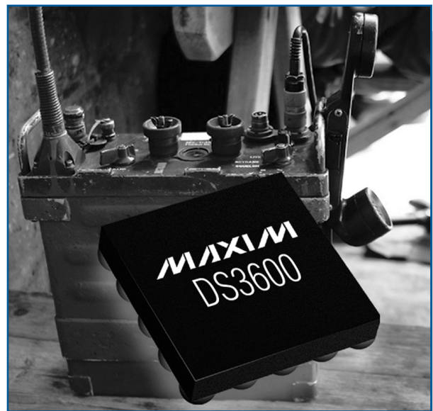
Figure 3. The CSBGA package of the DS36xx family provides a layer of passive protection by limiting access to I/O signals when the device is installed on a circuit board.
